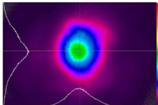
**Figure 10** Beam profile of 50 W regenerative amplification at 10 kHz repetition rate with 250 W pump power.
