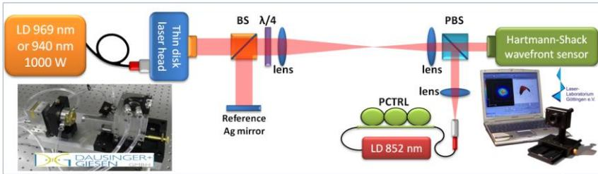
**Figure 8** Layout of the experimental setup (BS- beam splitter, PBS- polarized beam splitter, PCTRL- polarization control module).
