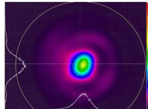
**Figure 17 Beam profile of 45 mJ Yb:YAG thin-disk laser output at 1 kHz repetition rate. Pump pulse duration was set to 500  $\mu\text{s}$  at 969 nm wavelength with pump power of 465 W.**
