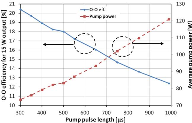
**Figure 11 Optical-to-optical efficiency (a) and required pump power to obtain 15 mJ output from Yb:YAG laser at 1 kHz (b) as a function of pump pulse duration. The average pump powers at each settings of pump pulse duration were adjusted so that the output energy was kept to 15 mJ.**
