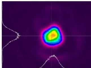
**Figure 9** Beam profile of a 102 W laser output in CW operation from an Yb:YAG thin-disk.
