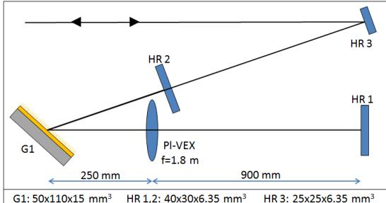
**Figure 6 Schematic pulse assembly introducing positive dispersion.**
