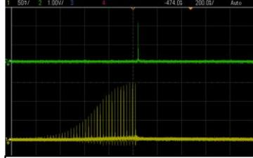
**Figure 18 Output pulse (top) and pulse build-up inside the cavity (bottom) of the regenerative amplification with an Yb:YAG thin-disk (time base 200 ns/div).**
