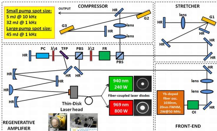
**Figure 3** Layout of the laser (OI-isolator, HR-high reflector, PBS-polarized beam splitter, TFP-thin-film polarizer, FR-Faraday rotator, PC-Pockels cell, G-grating,  $\lambda/2$ -half wave-plate,  $\lambda/4$ -quarter wave-plate).
