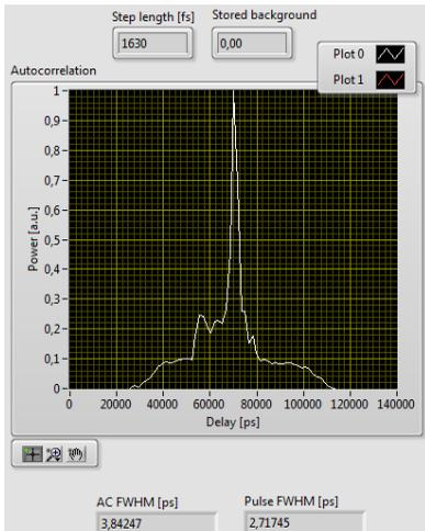
**Figure 19 Measured autocorrelation function of the compressed output pulse from a Yb:YAG thin-disk laser.**
