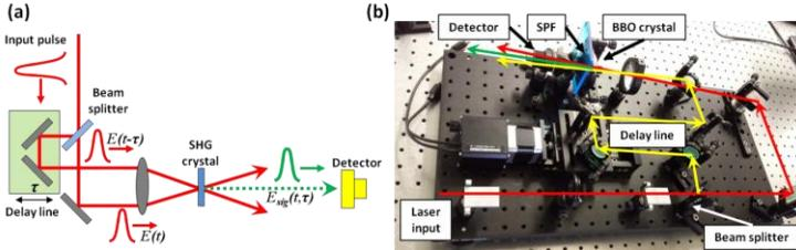
**Figure 2 Autocorrelator setup (a) and its laboratory realization (b) (SPF-short-pass filter, SHG second harmonic generation).**
