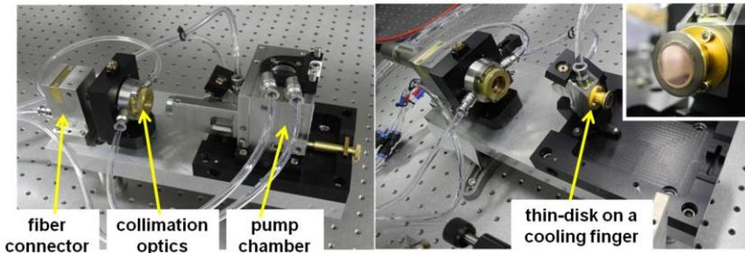
**Figure 4 TDM 1.0 Lab thin-disk laser module used in the regenerative amplifier.**
