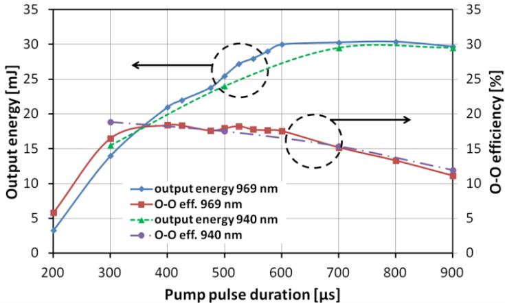
**Figure 21 Output characteristics of the Yb:YAG thin-disk regenerative amplifier operated at 1 kHz repetition rate pumped by two different pump wavelengths: 940 nm laser diode with a peak power of 265 W and 969 nm laser diode with a peak power of 285 W.**
