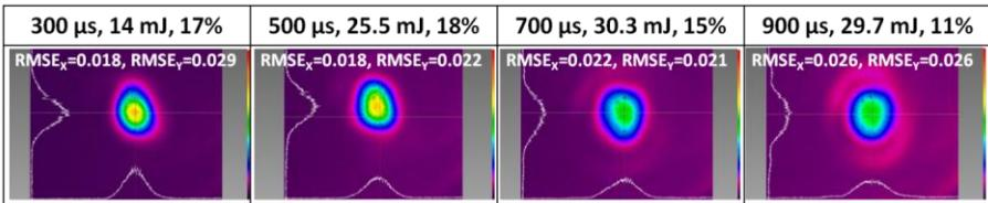
**Figure 16 Yb:YAG laser beam quality and O-O improvement for 969 nm pulsed pumping.**
