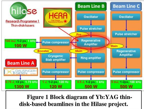
**Figure 1 Block diagram of Yb:YAG thin-disk-based beamlines in the Hilase project.**
