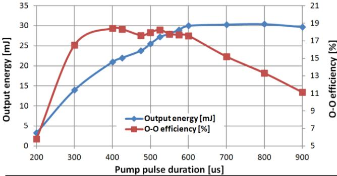
**Figure 15 Characteristic of the Yb:YAG regenerative amplifier pumped at 969 nm wavelength.**
