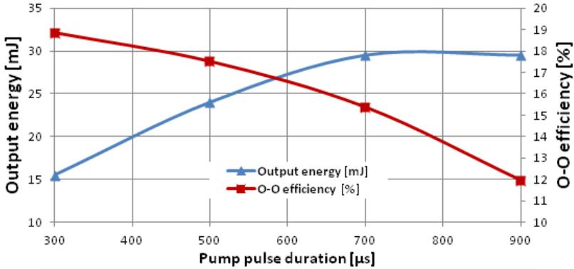
**Figure 13 Characteristic of the Yb:YAG regenerative amplifier pumped at 940 nm wavelength.**
