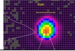
**Figure 12 Far-field profile of 10 kHz Yb:YAG regenerative amplifier.**
