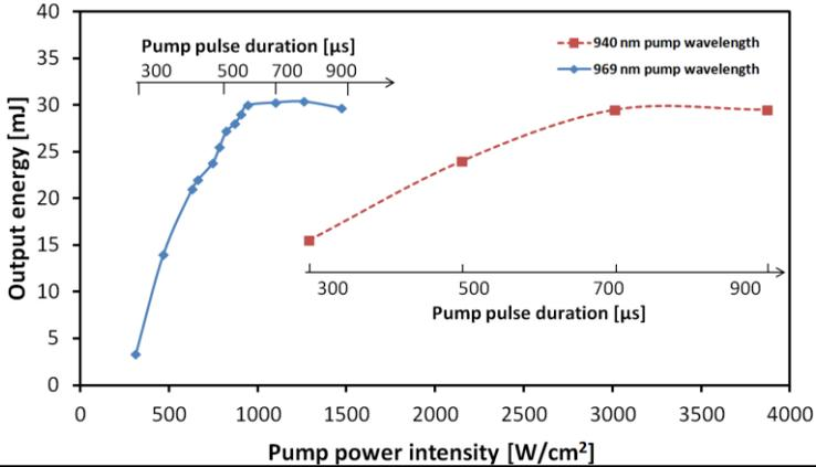
**Figure 22 Output characteristics of the Yb:YAG thin-disk regenerative amplifier operating at 1 kHz repetition rate for 940 nm pumping with a pump spot diameter of 2.8 mm and 969 nm pumping with a pump spot diameter of 4.8 mm.**
