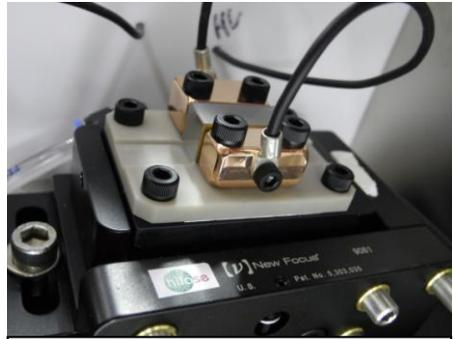
**Figure 5** Designed BBO holder with electrodes on a ceramic, water-cooled plate and 5-axis translation stage.
