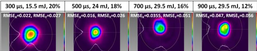
**Figure 14 Yb:YAG laser beam quality and O-O improvement for 940 nm pulsed pumping.**
