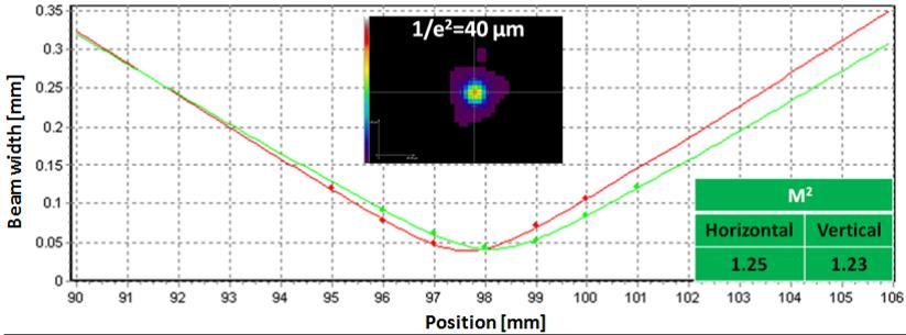
**Figure 20 Focusing property of the Yb:YAG thin-disk laser output pulse for the calculation of  $M^2$  value.**
